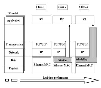
Fig.2.2 Classification of industrial Ethernet (IEC 61 784-2)
