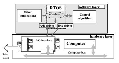
Fig.2.1. Hardware and software layers of the computer controlled system
