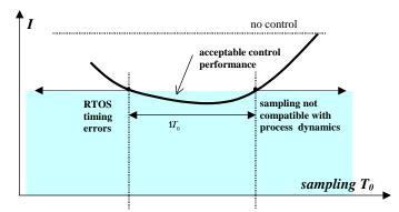
Fig.2.3. RTOS and process dynamic relations. For small  $\Delta T_0$  the control system becomes time critical. I – value of an objective function
