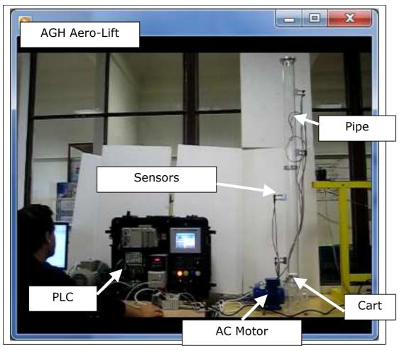
Fig. 5.2. Aero-Lift - laboratory test-rig
